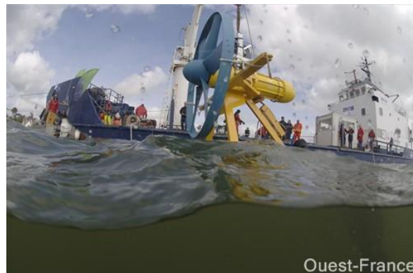
Figure III-8 : Hydrolienne prototype submersible Sabella [Gui 16,a]
